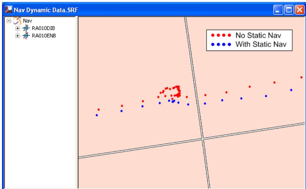
Figure 3-4 Plot showing results with static nav being applied verses no static nav
