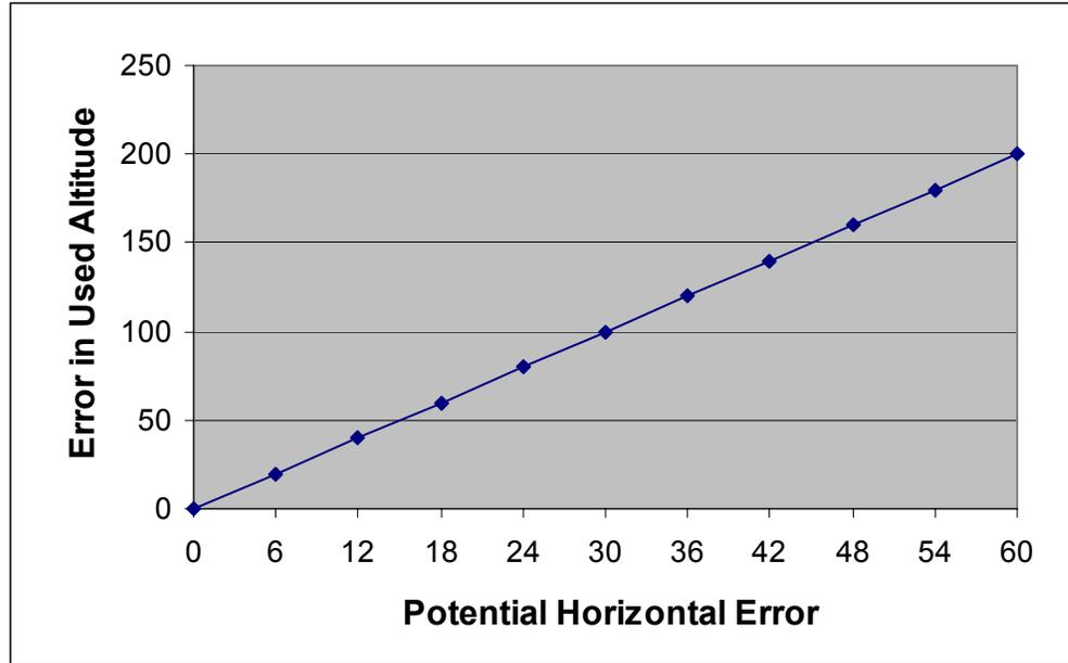
Figure 3-1 Potential horizontal error resulting from an error in the used altitude when operating in 2D mode
