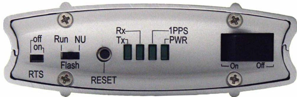
Figure 1-2 Front panel of the SiRFstarIII Evaluation Receiver
