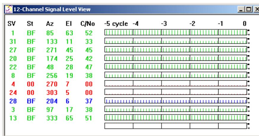
By using this screen, you can quickly see whether the receiver is navigating, how many satellites are being used, and the signal strength of each satellite. Table 4-2 lists each of the displayed values.
