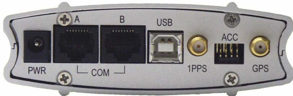
Figure 1-3 Rear panel of the SiRFstarIII Evaluation Receiver
