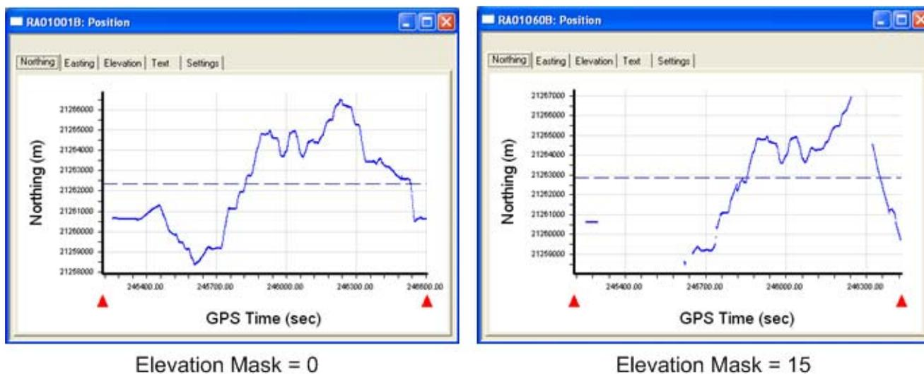
Figure 3-3 Results comparing a 0 degree elevation mask and a 15 degree elevation mask
