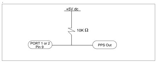
Figure 1-3 Open Collector PPS
