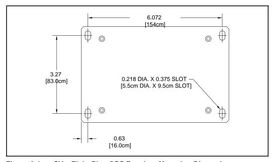
Figure 2-1 SVeeEight Plus GPS Receiver Mounting Dimensions
