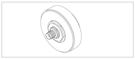
Figure 1-5 Hard Mount GPS Antenna
