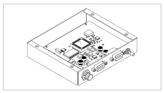
Figure 1-1 The SVeeEight Plus GPS with Bottom Flange Plate Removed Showing the Internal SVeeEight Board
